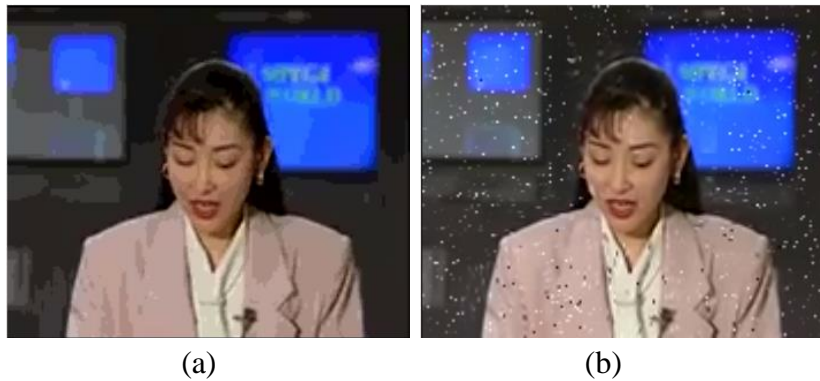
Figure 31. Video output with bit-truncation and voltage scaling. (a) Original video PSNR = 38.83. (b) Bit-truncation PSNR = 31.67.
