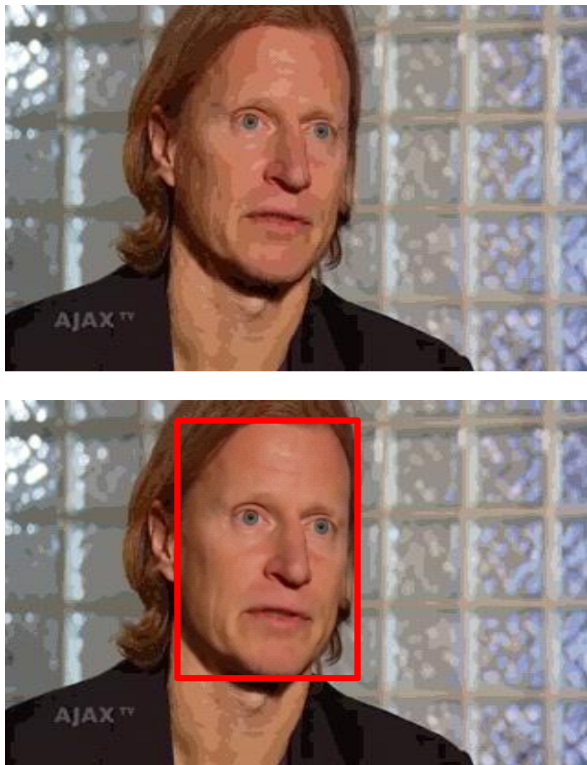
Figure 61. Top: 4 bits truncated; bottom: 4 bits truncated with 2 bits truncated in the detected face area.
