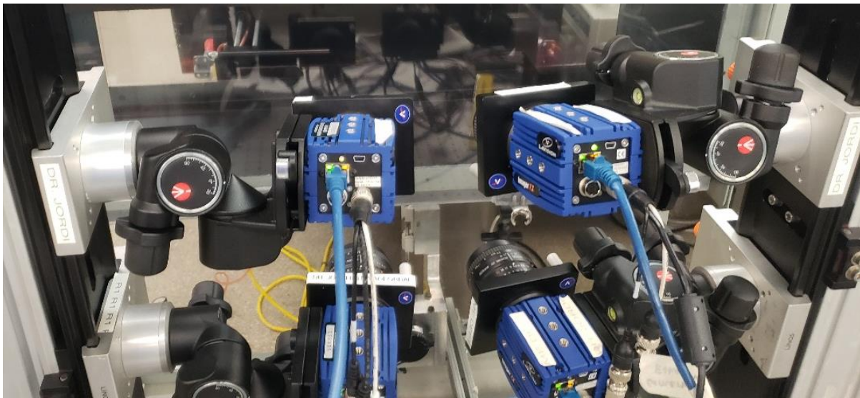
Figure 9: Camera Apparatus for Tomographic PIV
