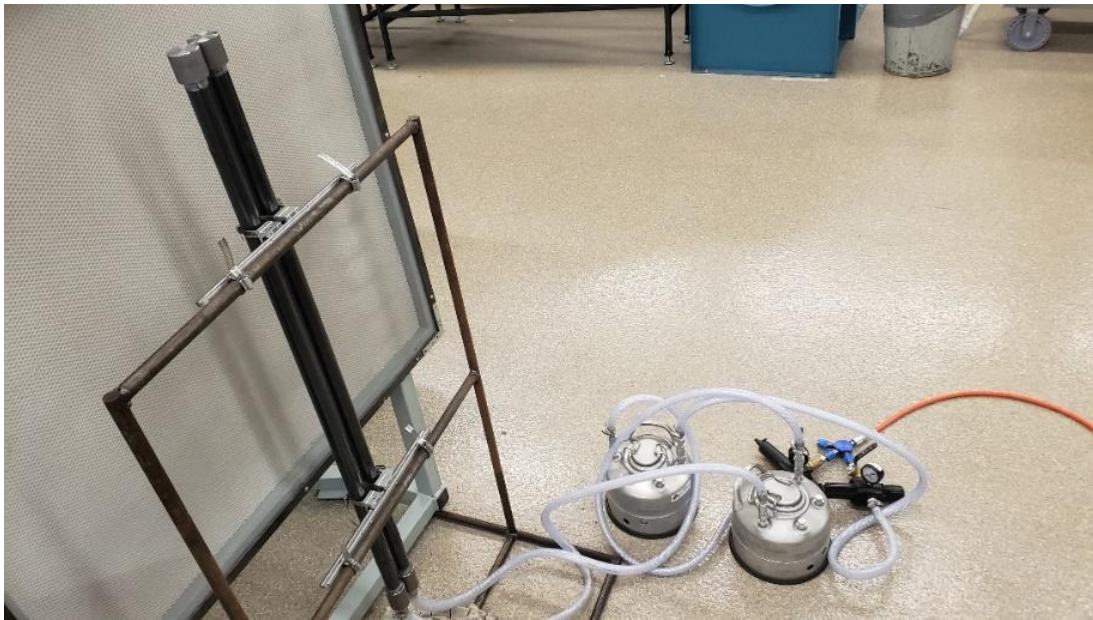
Figure 7: Wind Tunnel Particle Seeder Apparatus
