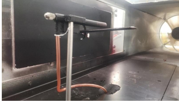
Figure 11: Vortex Generator Setup for Airfoil Interaction
