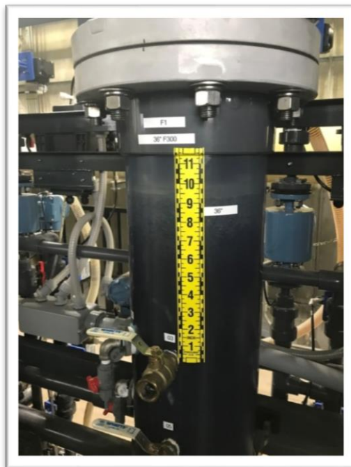
Figure A3: Photograph of Sample Ports of Column Loaded with GAC Within PFS System
