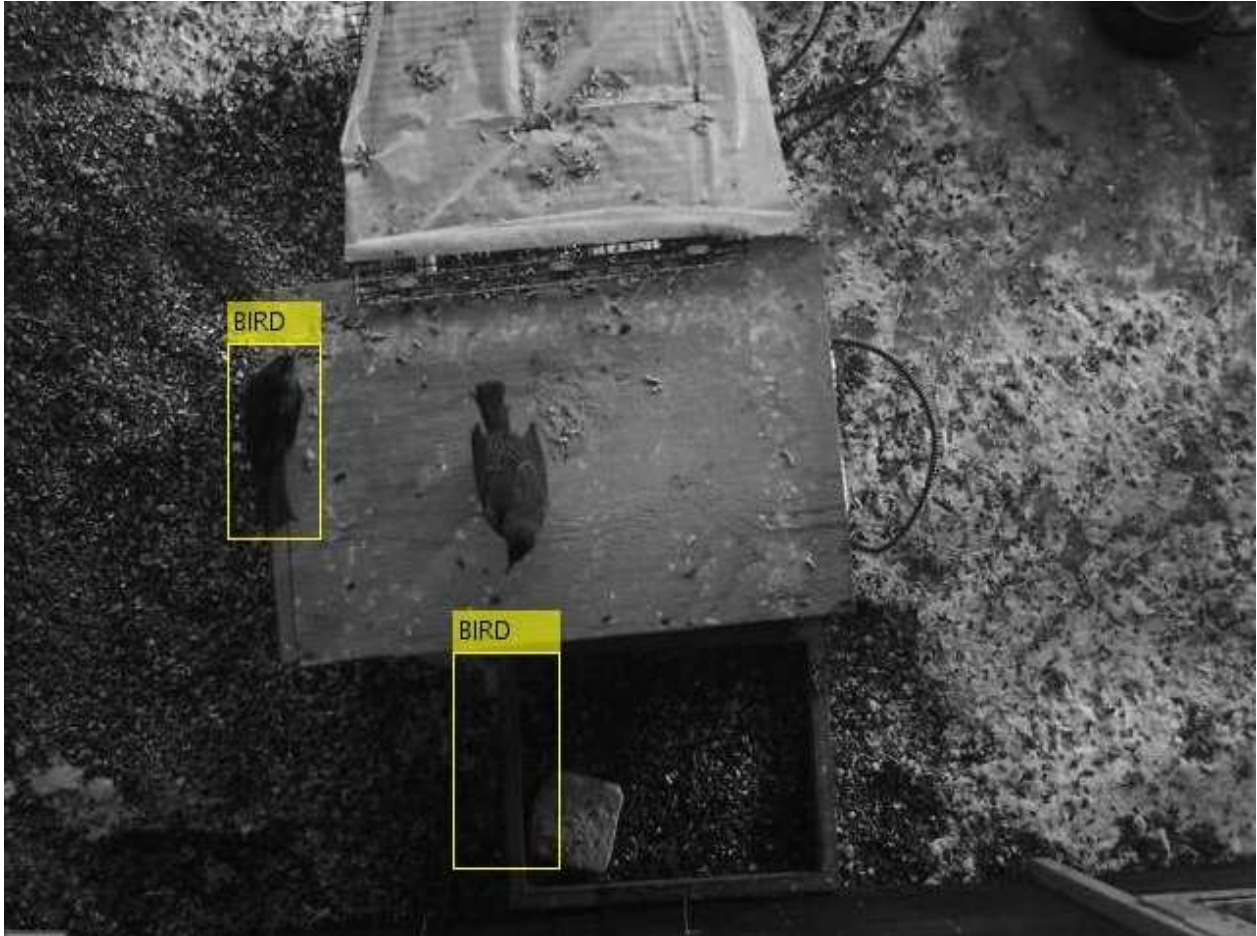
(b) Correctly Detected 0^\circ Aligned Bird with missed Rotated Bird and falsely Detected Bird, using VJA with no Rotation
