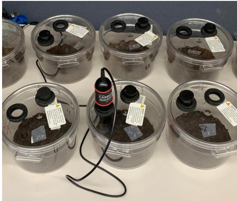
Figure 2. Biochamber used for the incubation of soil samples and CO 2 flux measurement for the study
