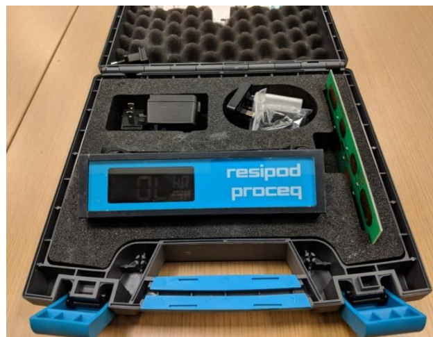
Figure 15: Electrical resistivity test equipment (Resipod Proceq)
