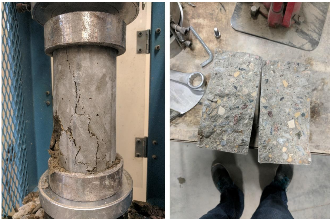
Figure 12: Failure of specimens during strength
