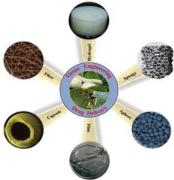
Figure 1.1. Different morphologies of silk processing (silkworm). Adopted from “chemically modified silk proteins; advanced engineering materials.”
