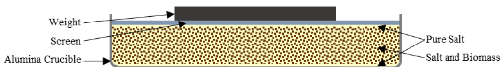
Figure 5.8: Cross sectional of the torrefaction apparatus
