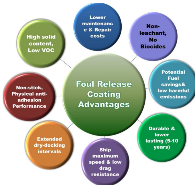
Figure 1.4. Economic and ecological advantages of fouling-release marine coatings. Reprinted from reference 62.
