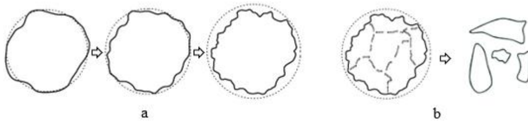
Figure 4. Suggested breakage pattern of black beans during single pass milling (a) Erosion and (b) Shattering.
