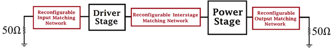
Figure 3.1. Macro-model of the proposed multi-band power amplifier using reconfigurable input, interstage, and output matching networks.
