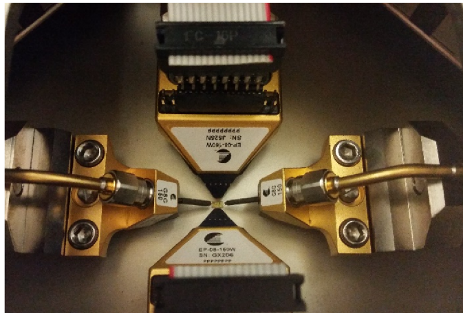
Figure 5.16. RF and DC probes used to characterize the BORN PA.
