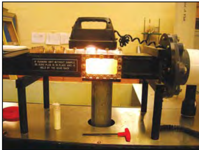
Measurement of Soil Erosion Rates using the Erosion Function Apparatus
