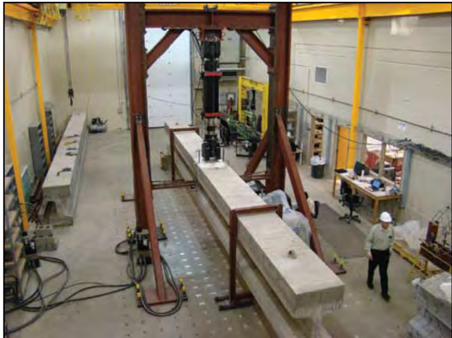
Testing on a Full-Scale Bridge Girder at the Lohr Structures Laboratory
