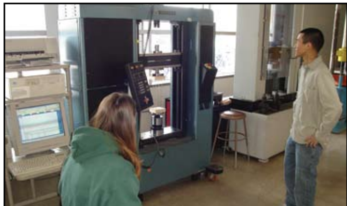
Jordan Jarrett and David Sawahata use an Instron testing machine to test a wood-dowel-based model to failure in compression. The models are a preliminary examination of using wood or biomass materials as flexible bending or compression members.
