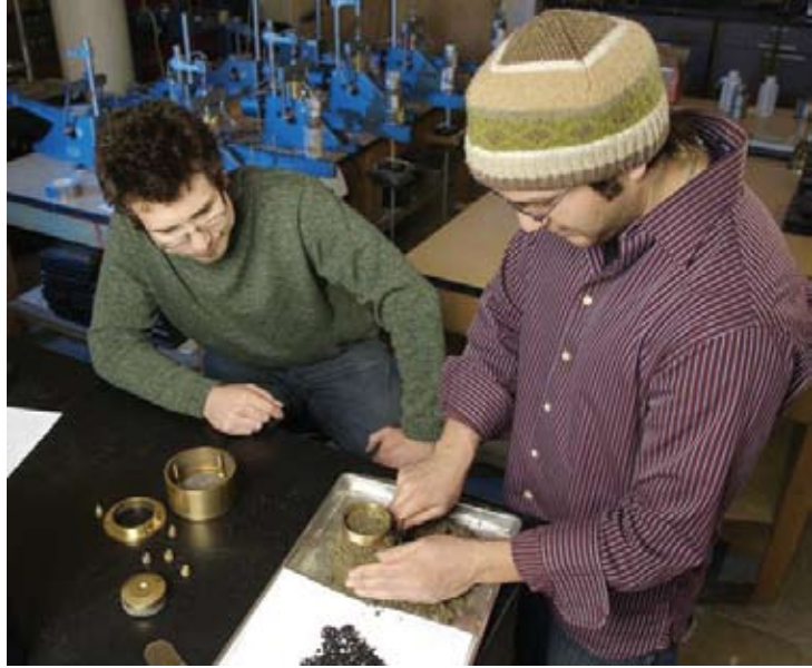
Research assistants Gabriel Iltis (left) and Jesus Higuera Seda (right) working on the preparation of specimens of expansive soil-rubber (ESR) mixtures for swell-consolidation testing.
