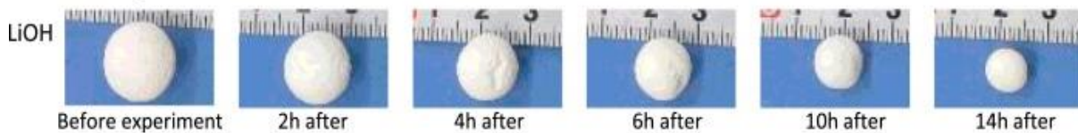
Figure 5. The change of phases of a lithium hydroxide compound during exposure to ethanol at 30^\circ\text{C} . [151]
