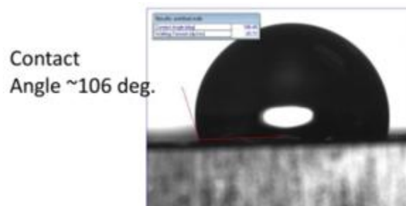
Figure 27. SLIPS Surface Exhibiting Hydrophobicity
