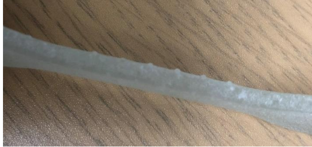
Figure 20: Dimpling on gauge section of tensile sample.
