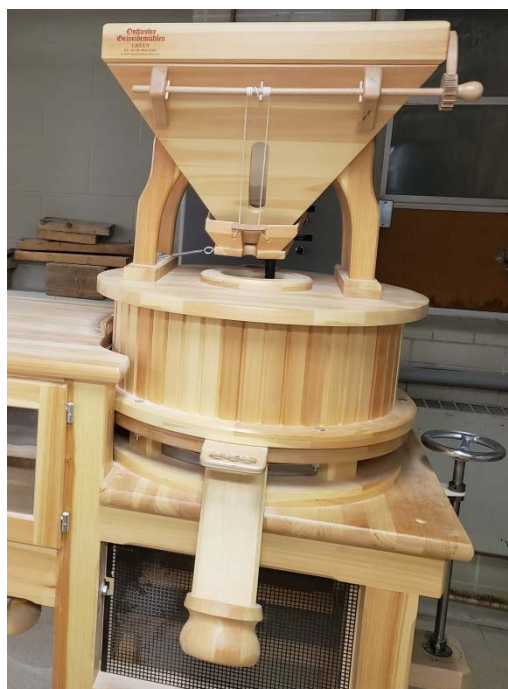
Figure 4. Stone mill model A 500 MSM and produced by Osttiroler Getreidemuehlen
