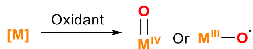
Scheme 1.2. Formation of high-valent oxo and oxyl species in the presence of metal complex and sacrificial oxidant
