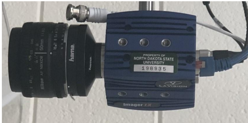
Figure 2.4. CCD camera used in the current PIV experiment.
