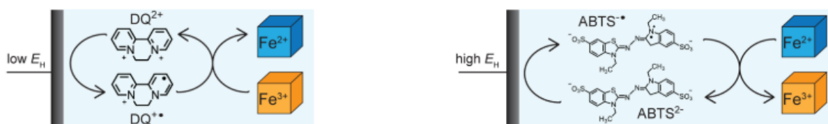
Figure 4.1. Electrochemical mediation of diquat and ABTS with iron ions. 5
