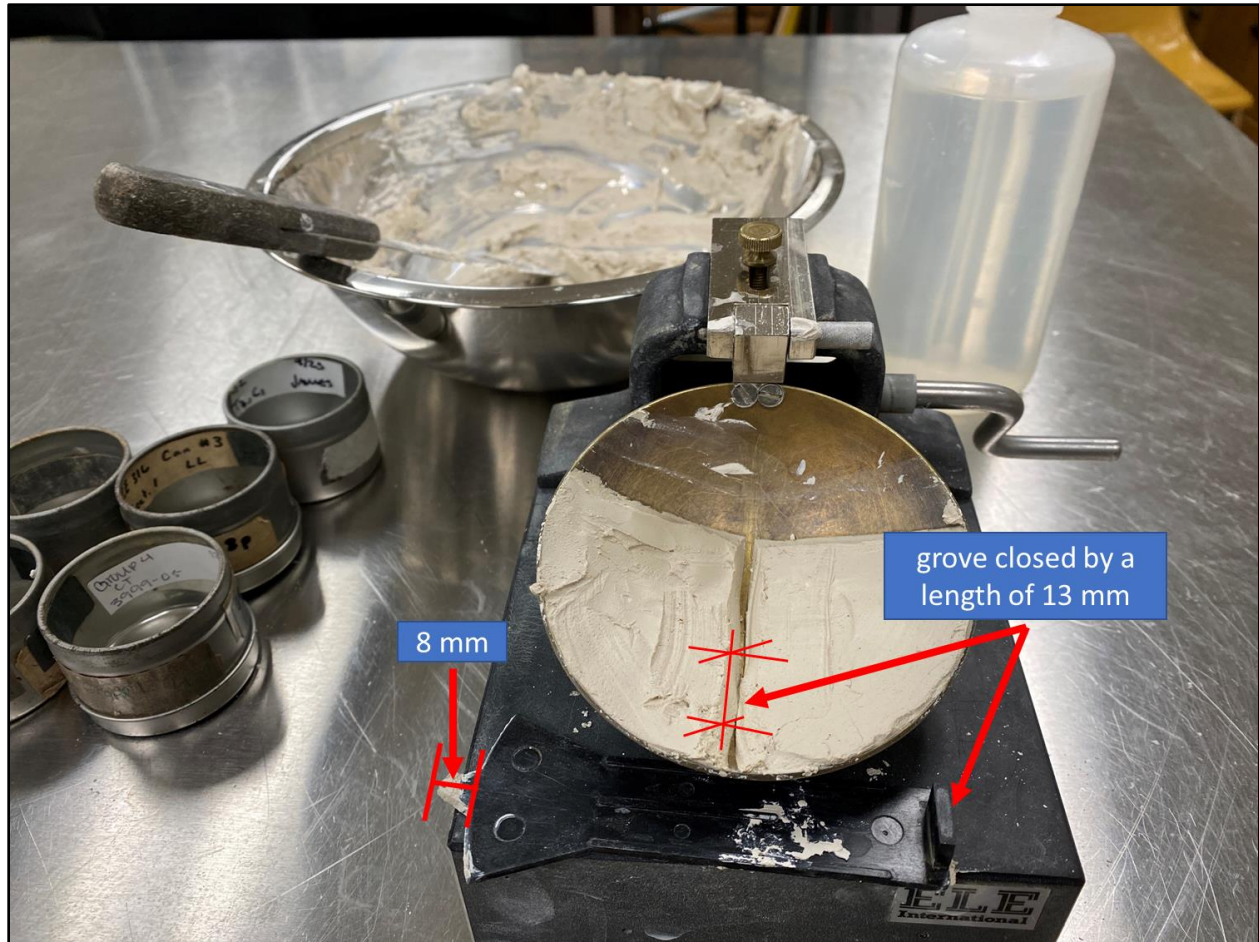
Figure 3.6. Liquid Limit Test in the Casagrande Device.
