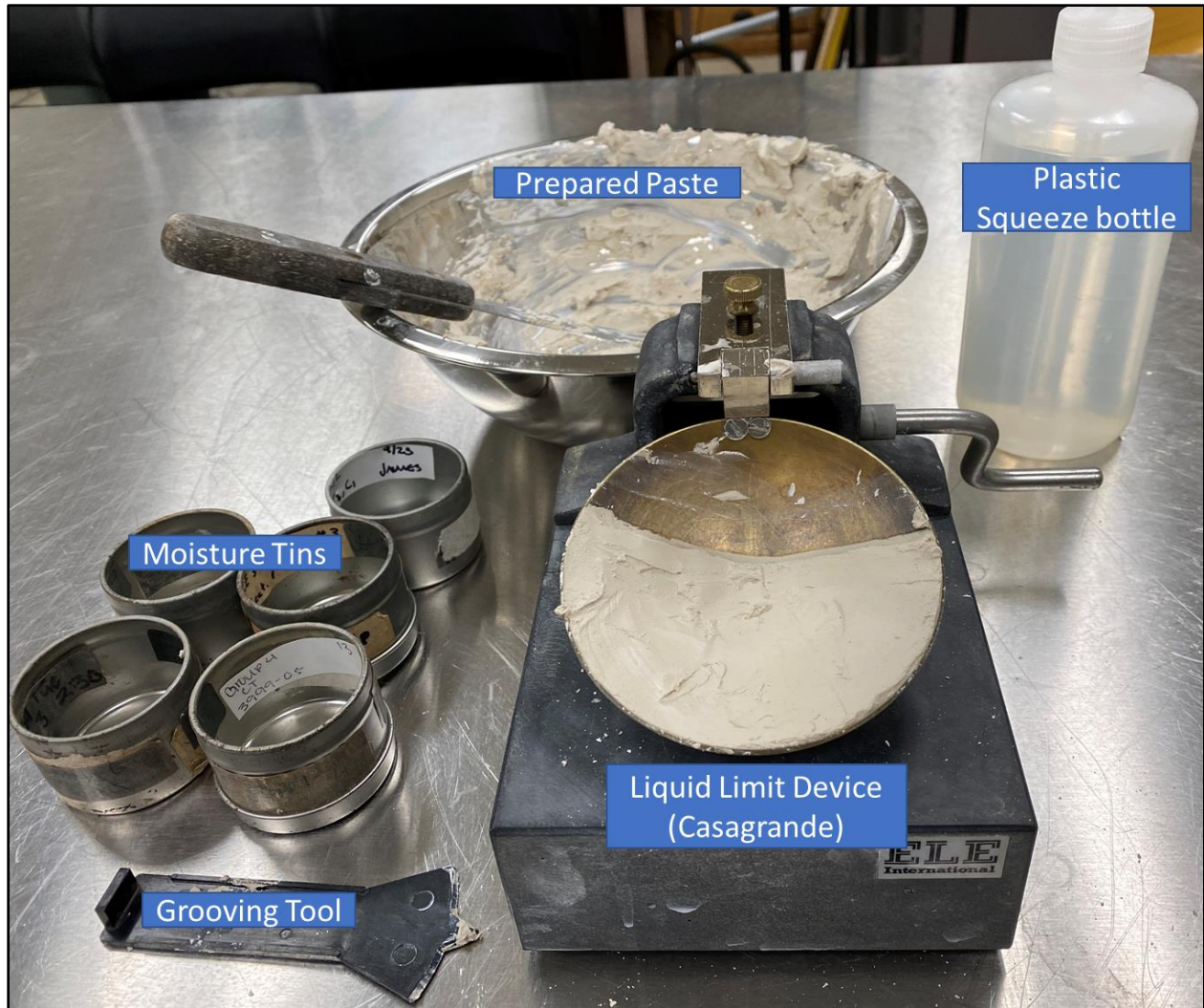
Figure 3.5. Sample Placed in the Casagrande Device for the Liquid Limit Test.
