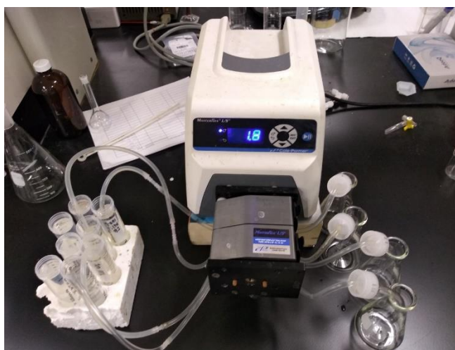
Figure 2.4: Pb (II) ions containing water solution passing through filtration device
