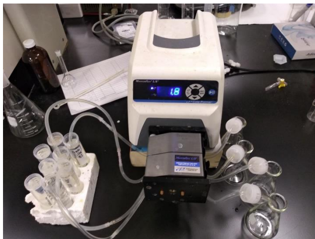
Figure 3.3: Pb (II) ions containing water solution passing through filtration device
