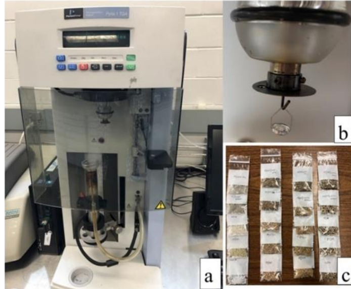
Figure 11. (a, b) TGA test set up (c) samples for the TGA test
