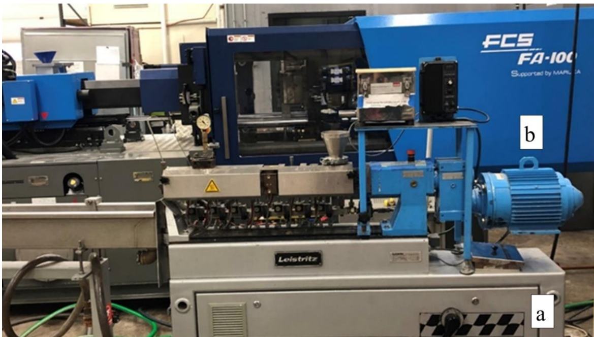
Figure 6. (a) Leistritz Extrusion and (b) injection mold
