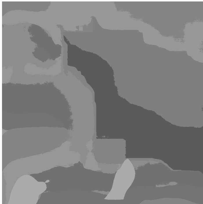
Figure 4.4. The output image from a cluster operation on a DEM file. Calculated with the following parameters: sum\_img\_size = 1000 , sub\_img\_start = [1000, 1000] , num\_clusters = 10 , average\_cluster\_values = True , analyses = [Analysis.slope, Analysis.aspect, Analysis.standard, Analysis.fractal, Analysis.fractal\_3d] , bands = [1, 1, 1, 1, 1] , and num\_agres = [7, 7, 7, 7, 7] .
