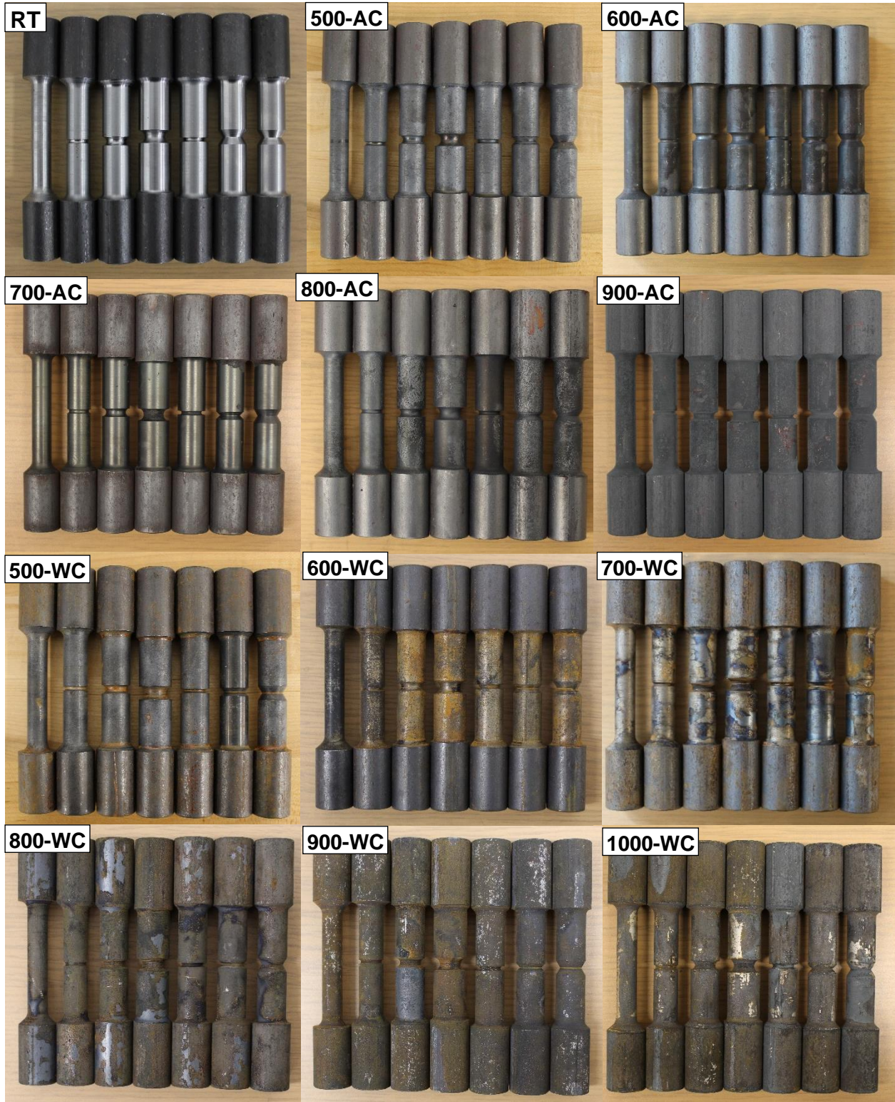
Figure 2.10. Specimens after being subjected to different temperatures and cooling regimes.
