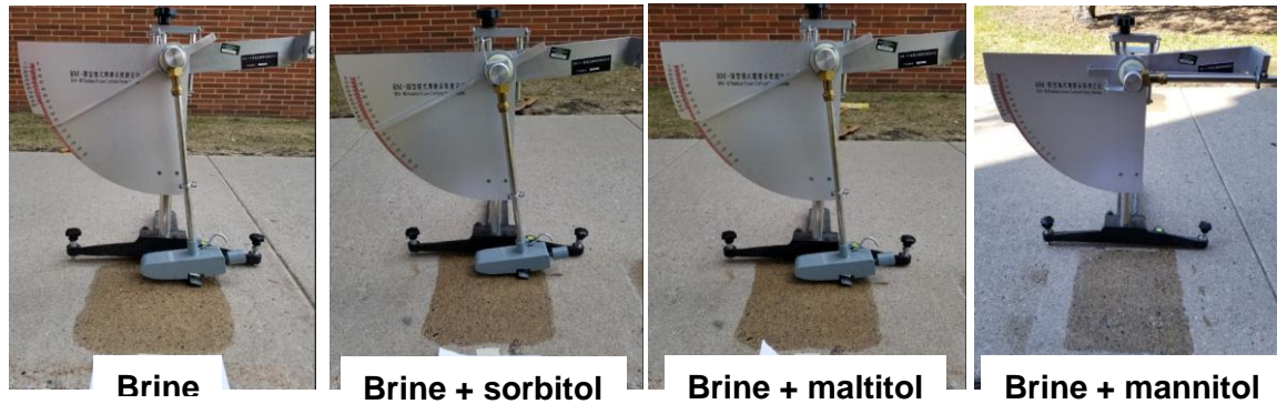
Figure 9.9. Skid resistance test on the PCC surface for all four optimal combinations of polyol and brine.
