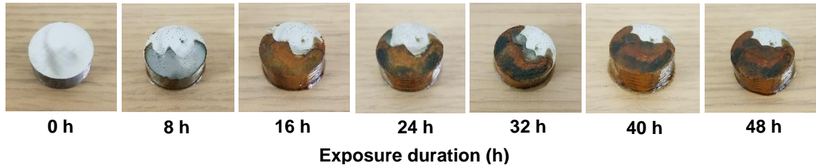
Figure 7.6. The visual appearance of ASTM A572 steel specimens exposed to the traditional deicing solution (23% NaCl brine).
