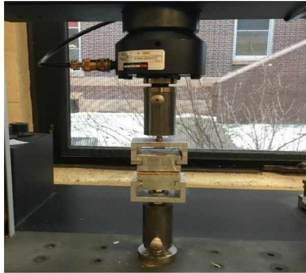
Figure 3.14: Internal bond test setup
