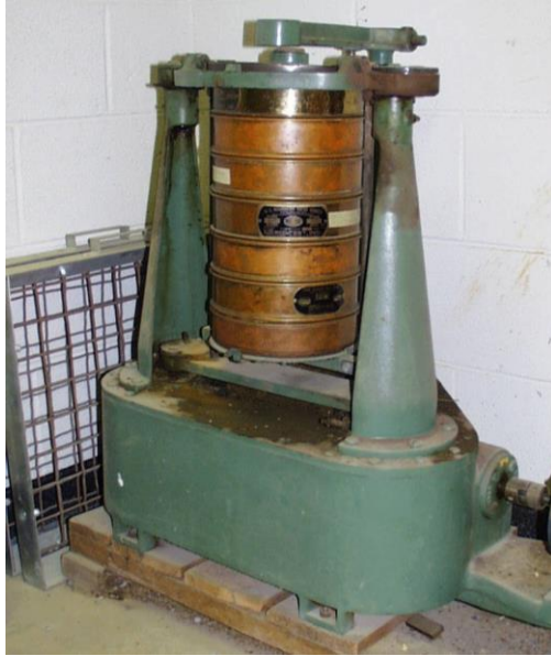
Figure 3.3: Sieving machine used for sieving DDGS and wheat straw
