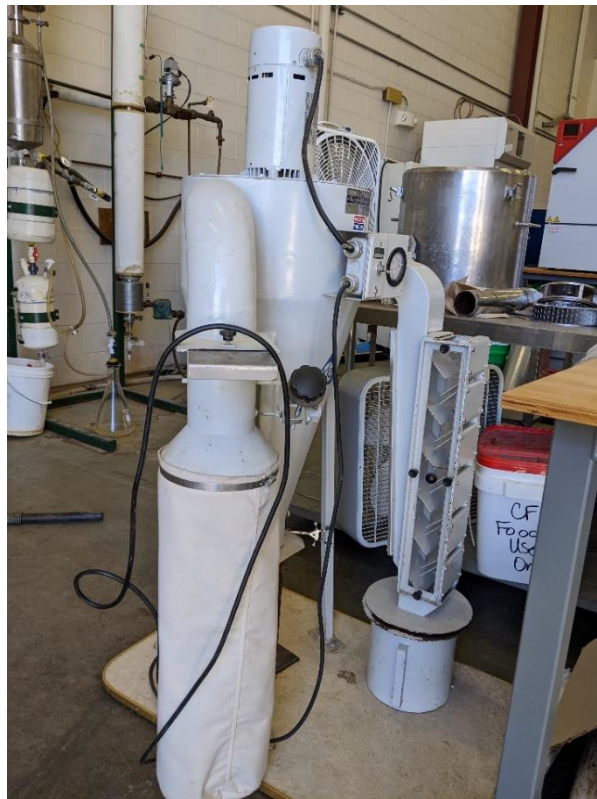
Figure 3.4: Air aspirator for fractionation of DDGS into heavier and lighter fractions
