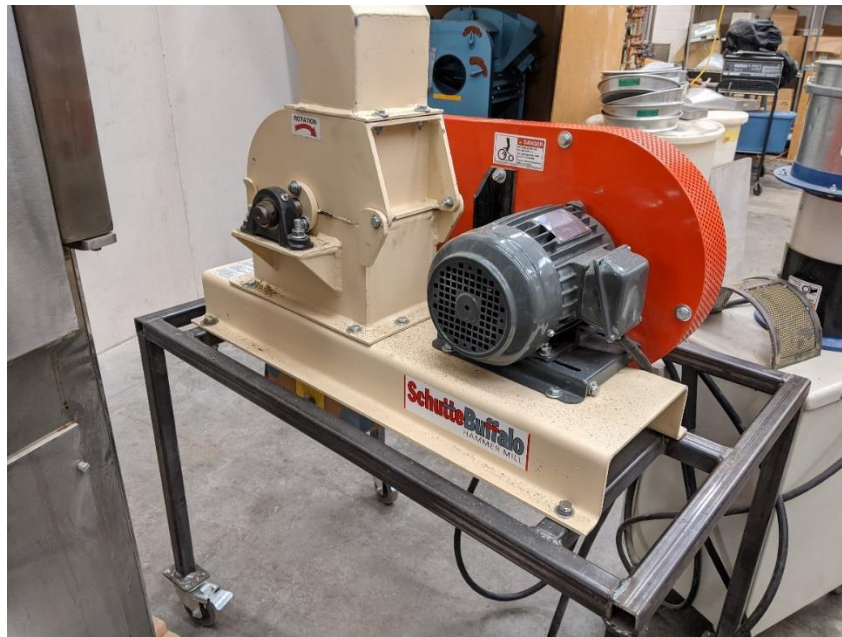
Figure 3.1: Hammer mill used for initial grinding of wheat straw
