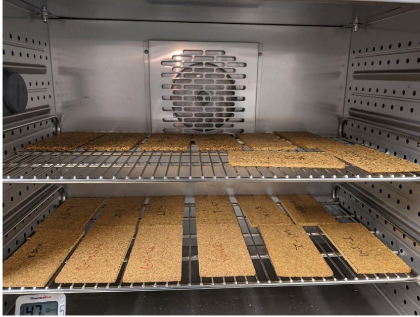
Figure 3.12: Linear expansion test samples arrangement
