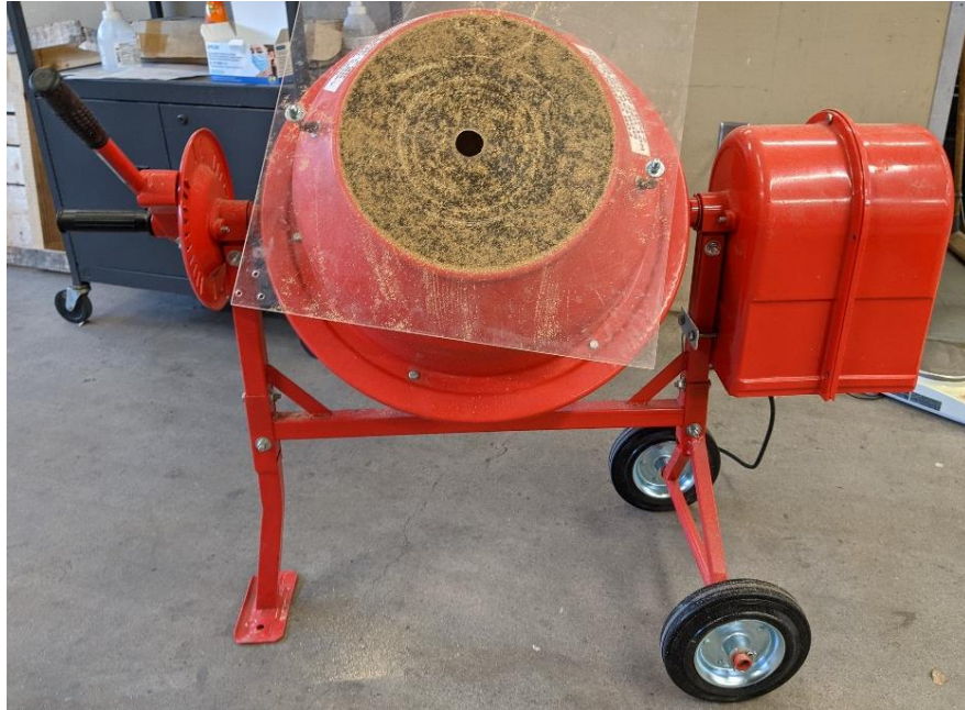
Figure 3.6: Cement mixture for mixing the raw materials with resin
