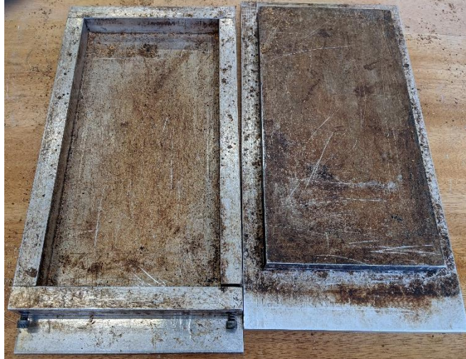
Figure 3.8: Mold for manufacturing particleboards
