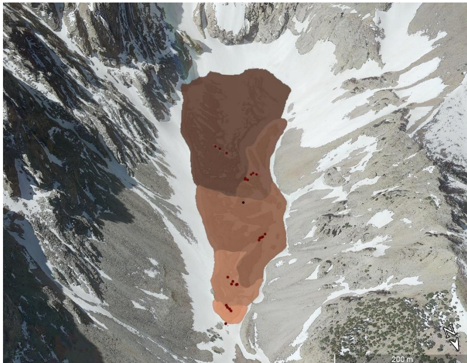
Figure 19. Topographic map of Wheeler Peak rock glacier with lobes highlighted by polygons graded from tan to brown. Red points mark boulders used in total station surveying, and the black point marks the take-off location for UAS flights. Satellite imagery obtained from Google Earth.
