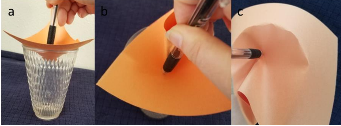
Figure 3. In figure a. and b. show the formation of a D-cone by applying a force in a small area on a sheet. This sheet is then pressed through a round opening forming the D-cone. In c. a heavy sheet is used, as the force pushes the sheet through the round opening D-cones are also formed along the edges of the opening; the sharp points seen in the picture.
