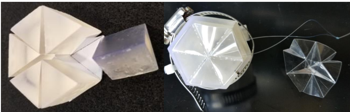
Figure 54. 3-D printed apparatus for the triangle origami pattern. Where the 3-D printed structures are placed triangle side down onto each triangle and then pushed together to create a load holding the pattern in the “on” configuration.
