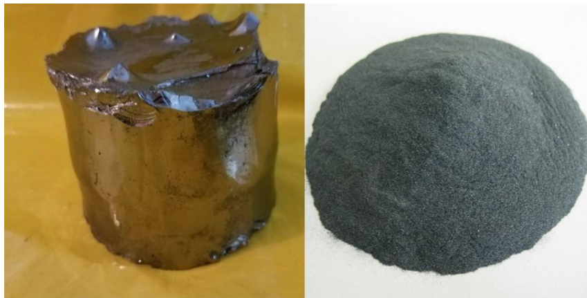
Figure 1. Left side: A bulk single SiC crystal originally made by Texas Instruments that has yet to be sliced into SiC wafers. Right: Granular SiC 180-grit powder used as an abrasive. Images used with permission from eBay sellers lo-so59 and iain4670, respectively.
