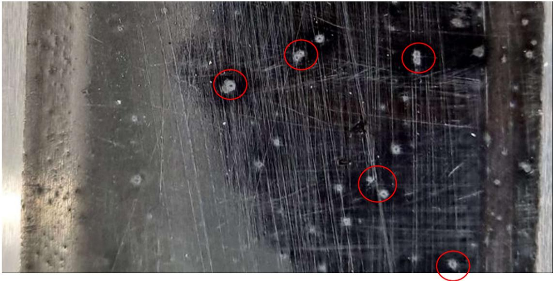
**Figure 5.2:** Visible agglomerates present in the CNT samples (sample shown is intentionally abraded)
