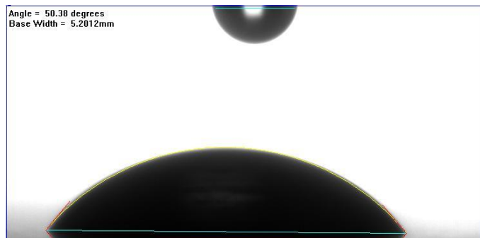
Figure 45: The image of contact angle measurement. A drop has a volume of 10\mu\text{l} and lays on the Ti13Nb13Zr surface with surface roughness less than 5\mu\text{m} .
