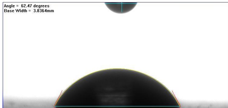
Figure 49: The image of contact angle measurement. A drop has a volume of 10 \mu l and lays on the Ti13Nb13Zr surface with surface roughness between 31 to 36 \mu m.
