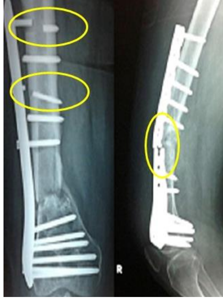
Figure 12: X-ray graph of Mechanical failure in orthopedic implant [251].
