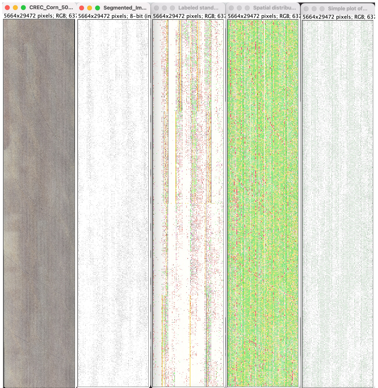
Figure 3.12. Field-scale demonstration of the developed stand count plugin showing original, binary, stand count, spatial distribution, and simple plot of plants. The field dimensions are about 146 ft wide by 760 ft with an area of 2.6 ac.
