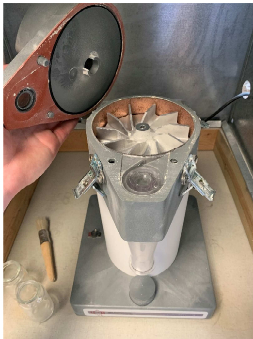
Figure 4. UDY cyclone mill prior to milling
