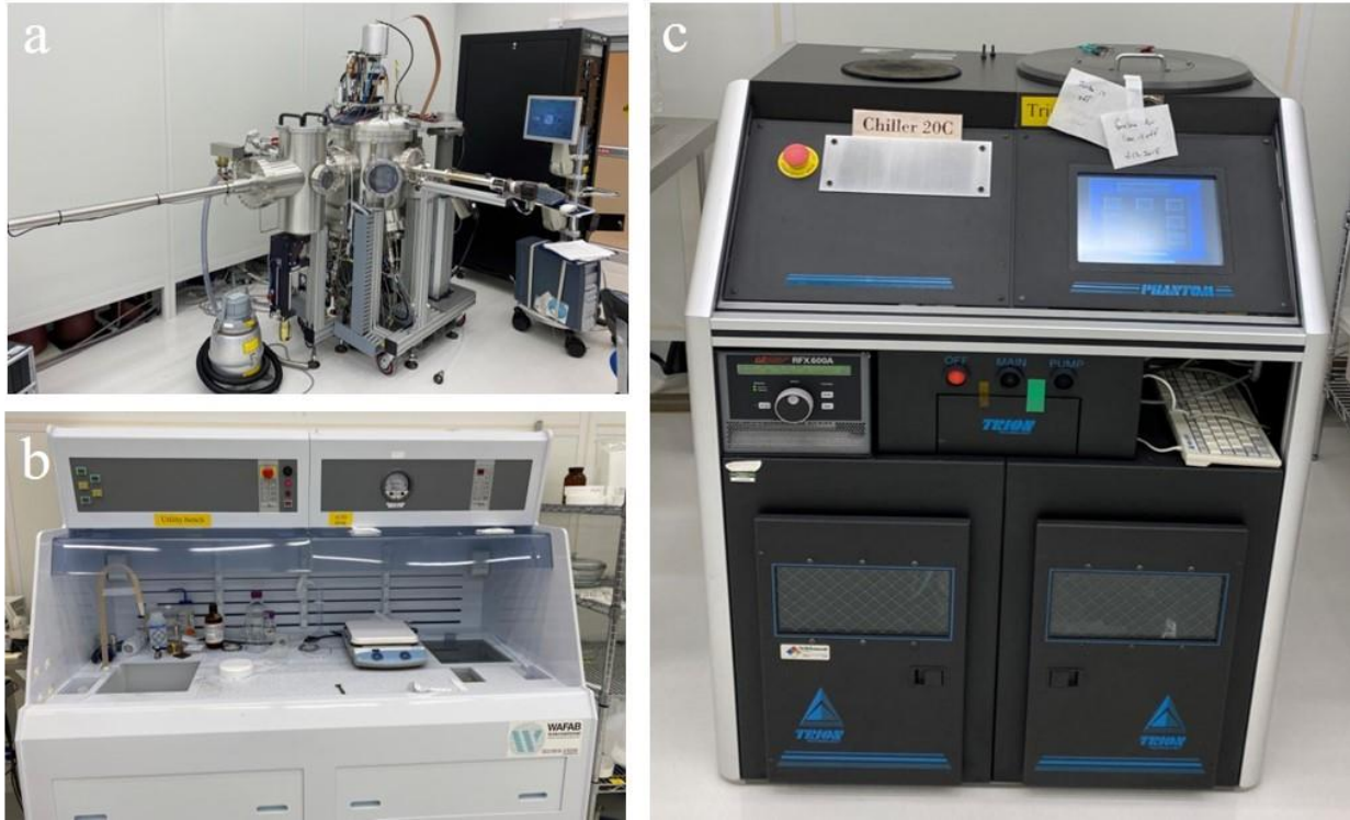
Figure 49. Instruments for microfabrication in a cleanroom. (a) Kurt Lesker CMS-18 sputter for aluminum deposition. (b) Utility bench. (c) Trion RIE plasma etcher.
