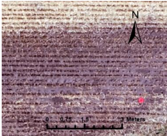
Figure 2. Detail of the UAS imagery from the study location showing the known ground control point used to georeference the prescription maps. Orange plastic lid used as reference for the southeast corner of prescription map and south edge of sprayer boom. Imagery collected by a DJI Phantom 4 RTK at 76 m [249 ft] AGL at the Carrington Research Extension Center, Carrington, ND.
