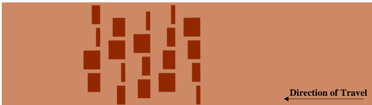
Figure 4. Prescription map generated by ArcGIS for AgLeader SMS for pass 2. Showing the length study (4 treatments and 5 replications) at the speed of 13.5 km h -1 . Light color =0 gal/ac and dark color =15 gal/ac.
