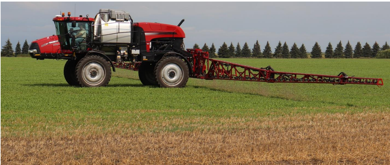
Figure A2. Case Patriot 4440 self-propelled sprayer applying red dye solution during the initial trial. Photographed at CREC.
