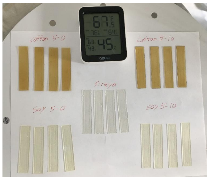
Figure 19. A variety of DMA bars conditioning in an atmospheric chamber.
