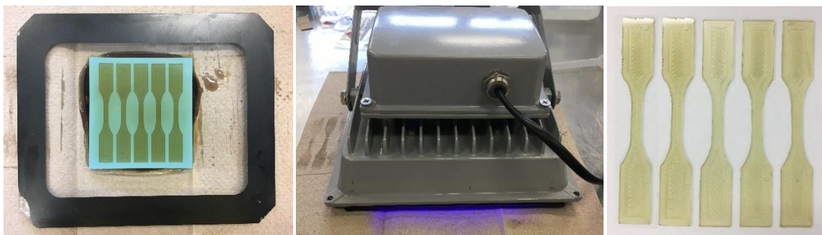
Figure 18. Manufacturing procedure for tensile samples.
