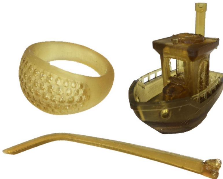
Figure 24. 3D printed ring, Benchy, and glasses temple models with 55% AECO formulation.
