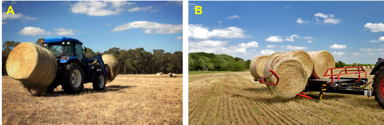
Figure 3.1. Examples of common and modern bale aggregation equipment: (A) Tractor equipped with bale spears at the front and rear (capacity = 1–2 bales); and (B) An automatic bale picker (ABP) with loading arm (capacity up to 23) — Image sources: https://www.himac.com.au and https://www.farm-king.com .
