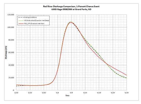
Figure 4 Effect of Diversion Inlet Gates on Hydrographs at Grand Forks, ND
