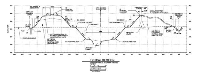
**Figure 5 Diversion Cross-Section Changes**
