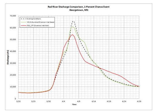
Figure 2 Effect of Diversion Inlet Gates on Hydrographs at Downstream End of Diversion Channel
