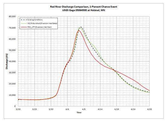
Figure 3 Effect of Diversion Inlet Gates on Hydrographs at Halstad, MN
