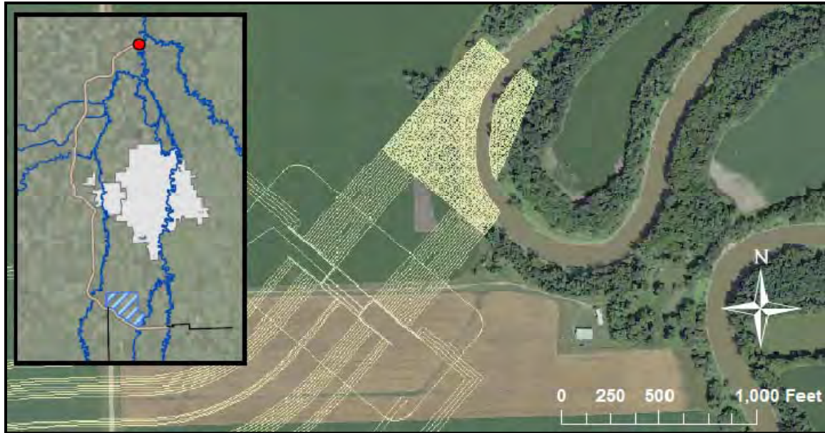
Figure 87 - Potential footprint impact area on the Red River for the downstream weir at the confluence with the flood diversion, North Dakota diversion alignment. The Minnesota diversion alignment would join the Red River at a different location, but would have similar characteristics.
