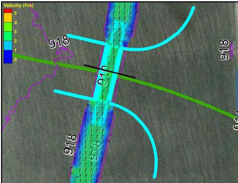
Figure 103 - Average velocities for the Maple Aqueduct under the LPP for a discharge equal to a 2-year event.
