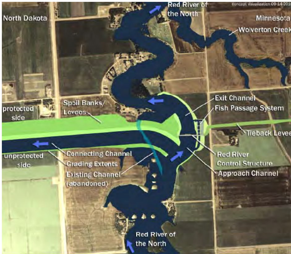
Figure 31 – Red River Control Structure visualization with flooding.
