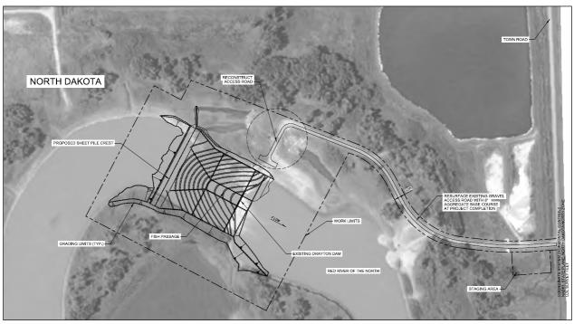
Figure 4. Proposed Drayton Dam fish passage alternative on the Red River of the North. Design and aerial photo are rotated so that the "west" direction is straight up; "north" is directly right.
