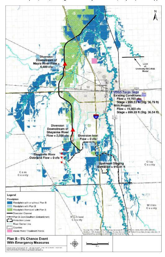
During the 21,000 cfs to 39,000 cfs operational range, a maximum of 20,000 cfs would be allowed through the DIS into the Diversion Channel. The gates on the DIS would be operated to limit flow increases to 2,000 cfs per hour. This operational limitation is intended to minimize potential for erosion within the diversion channel. The maximum surface water elevation in the staging area during this operational period, which includes the 100-year flood event, would be 921.0 feet (Illustration 3-2).
