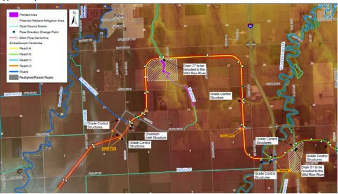
On the Minnesota side, the Dam/Southern Embankment has been realigned such that it follows relatively high ground from the Red River to Highway 75. Then, it extends south to a location
