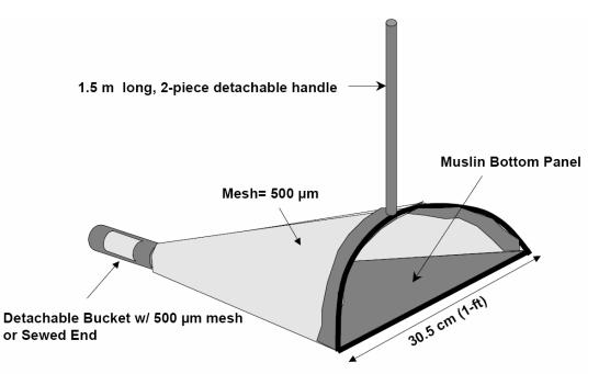
Figure 7.17.1. Modified D-frame Kick Net (Not drawn to scale)
