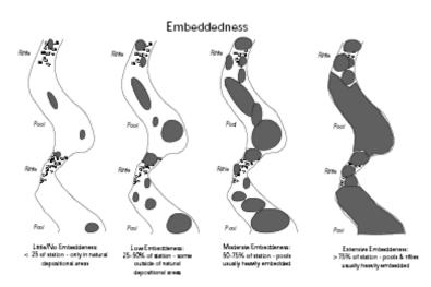
Figure 8. Illustration of example of degrees of pervasiveness of embeddedness for this QHEI component.
