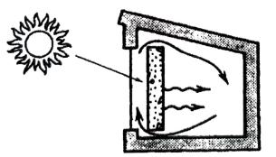
Isolated gain traps heat from the sun in an intermediate space.
