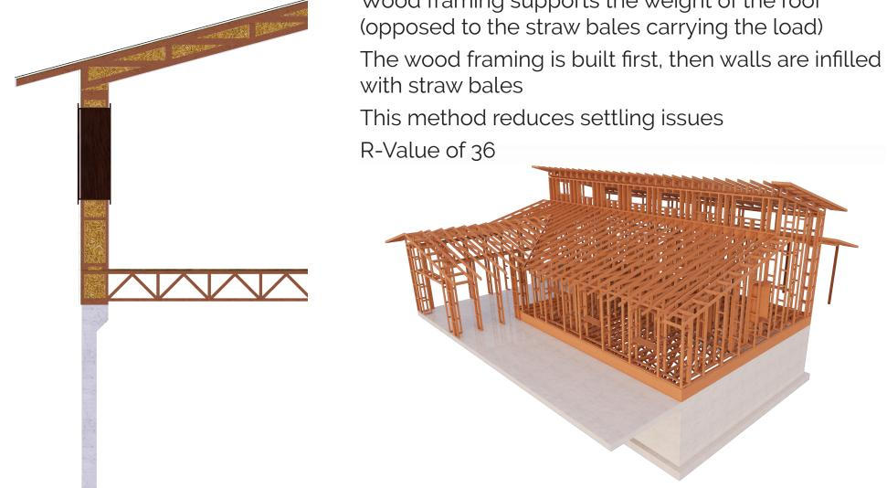
Wood framing supports the weight of the roof (opposed to the straw bales carrying the load)
