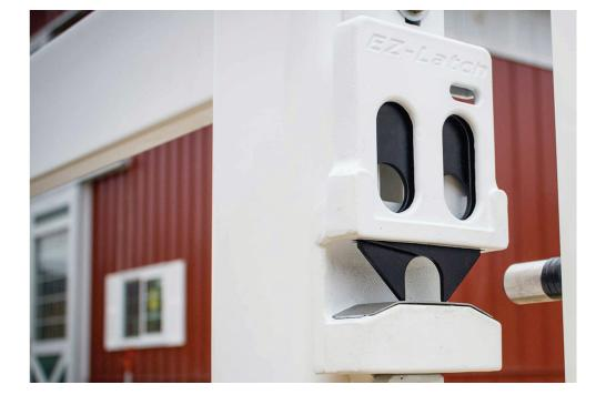
Two-way self-closing gate latches allow for gates to swing both directions and can be latched by simply swinging the gate shut. This makes opening and closing gates quick and easy while also ensuring that they are secure.
