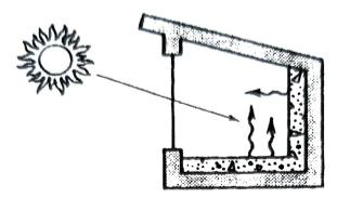
Direct gain uses heat from the sun that comes directly in to heat a space. This is most commonly achieved by placing large windows on the south facade.
