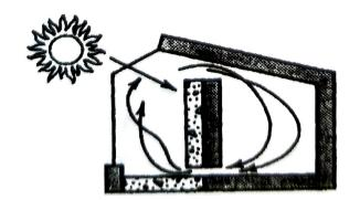
Thermal mass uses a large mass to capture heat during the day and radiate it into the space at night, Thermal masses can also be used during the summer to cool the space.
