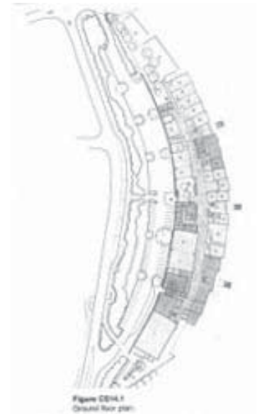
Figure 62. Ground floor plan showing relationship of building to road as well as organization of rooms.
