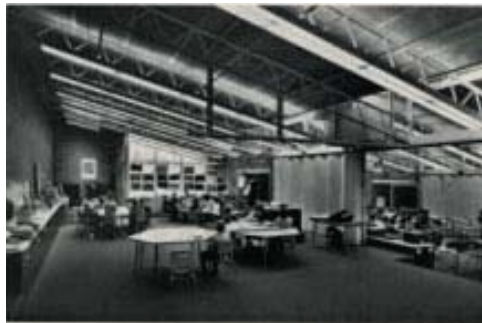
Figure 60. Clerestory windows allow light to flood deep into the classrooms which are essentially large open spaces.
