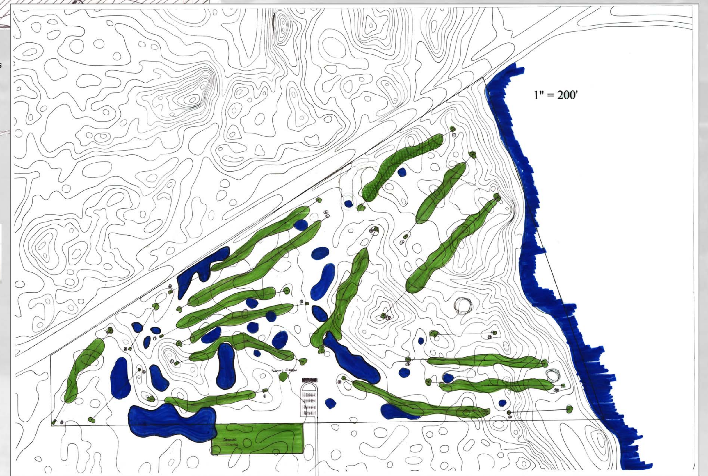
Beginning to finalize master plan by measuring the length of the holes and the water capacity of the ponds. Parking lot and clubhouse square footage measured.
