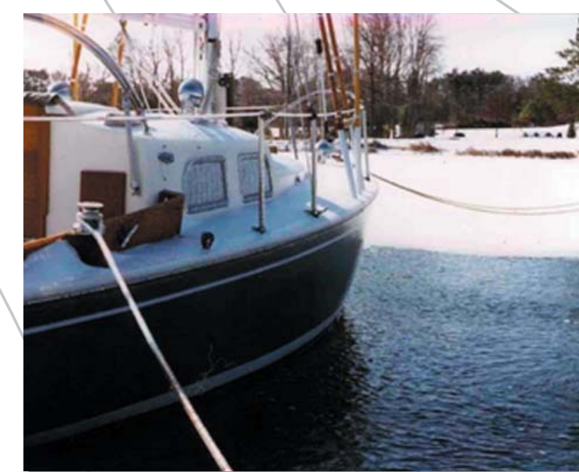
Bubble system combats ice formation around.
