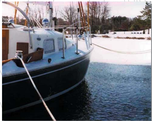
Bubble system combats ice formation around.
