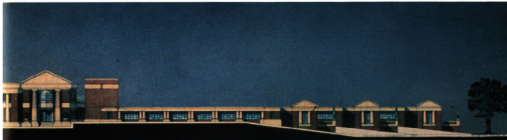
NCPA building, right and below, isolates mechanicals in a separate building (left) from lab spaces.
