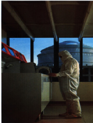
Above and top, MIT's microsystems technology lab is an adapted building housing clean rooms up to Class 10.
