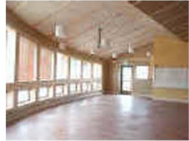
Figure 5.4. Emphasis put on day lighting and operable windows for natural ventilation, reducing energy consumption
