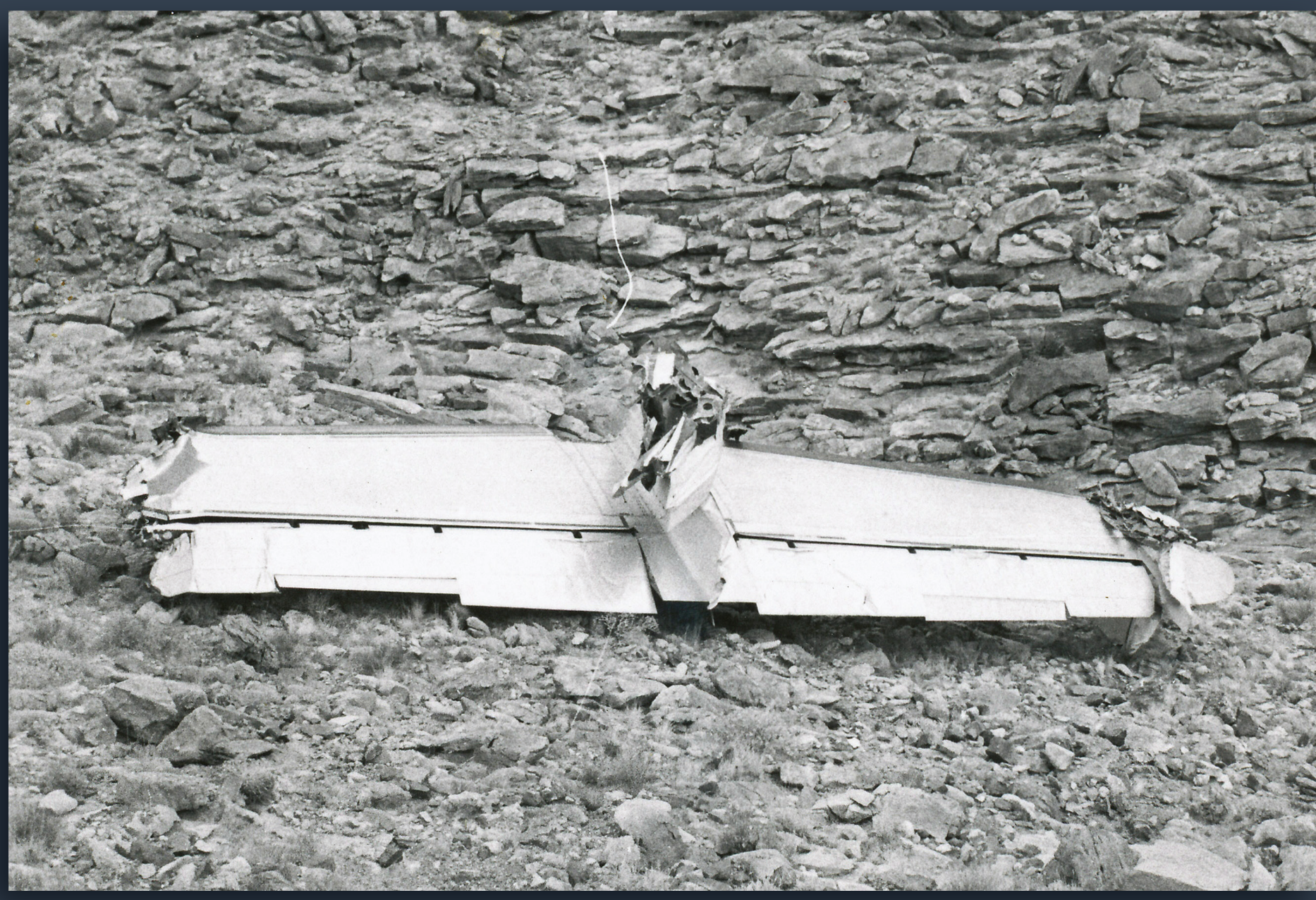
The scattered tail assembly of the TWA Collision with the unique three vertical stabilizers missing, as photographed by park rangers during the CAB investigation. | Courtesy of the National Park Service
